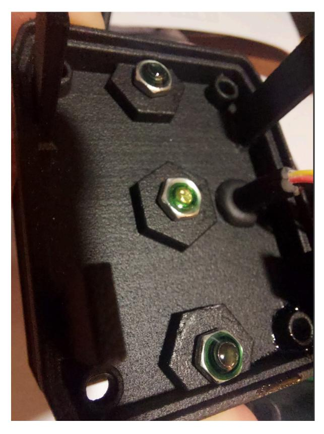
Once the loc-tite has cured, carefully close the box, making sure that the internal signal wires are comfortable. Screw the four M3 screws into position to secure the LED box backplate. Do not overtighten.
