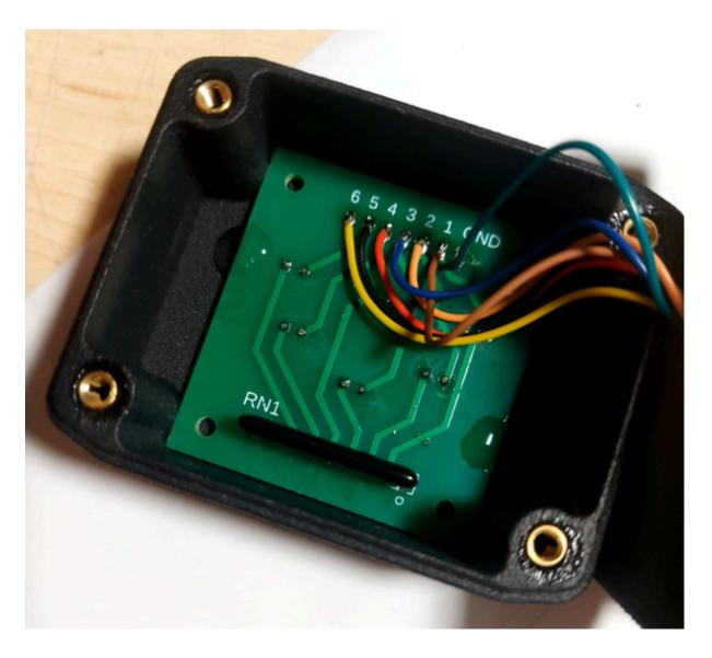
Turn the circuit board over and trim any protruding resistor legs and signal wires close to the board to prevent them from creating a space between the circuit board and the 3D printed case. The circuit board should sit close to the 3D printed case. Aim for a gap no larger than 1.5mm.
