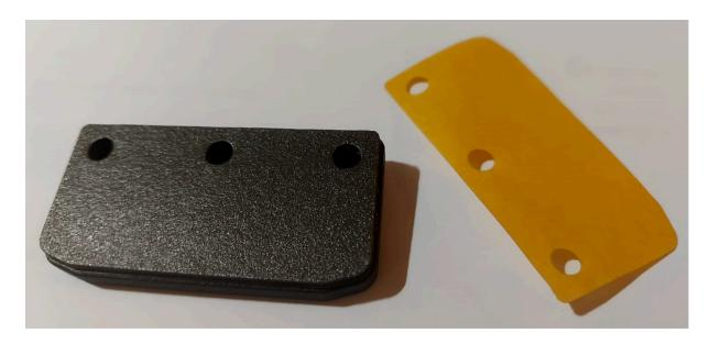
Place the two black M4 socket screws into the outer two holes (the screws are inserted from the plastic side, not from rubber side) and screw one M4 nut onto each. Leave approximately 6mm of thread exposed.
