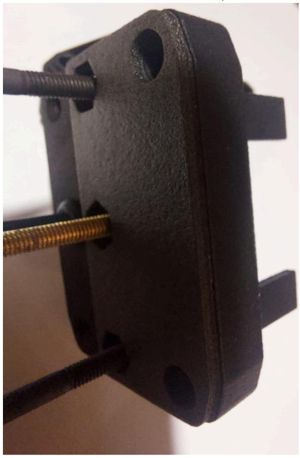
Screw M4 nuts onto exposed thread inside LED box and tighten these nuts against the first set of nuts. This is easier to do with a 3mm Allen key, and a small adjustable spanner. It is important that the nuts on the brass bar are tight. Once tightened, place a small drop of loc-tite or acrylate super glue onto the nuts inside the LED box and leave to cure.
